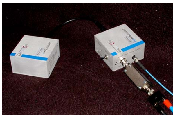
Figure 11b: Connection of the battery pack to the transmitter
