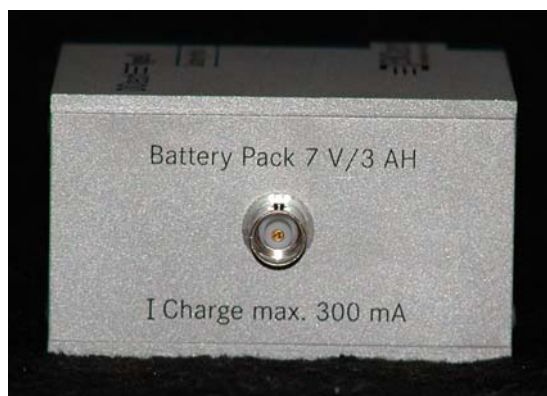
Figure 11a: Battery pack
