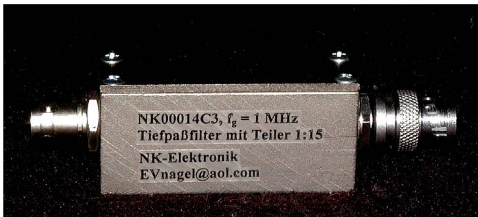
Figure 5: Low pass filter with integrated divider
